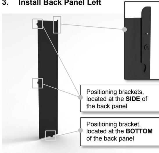
Place the positioning bracket at the bottom of the back panel in the horizontal groove of the NETpodium profile.
