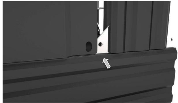
Make sure that the back panel is positioned in front of the installed bracket.
