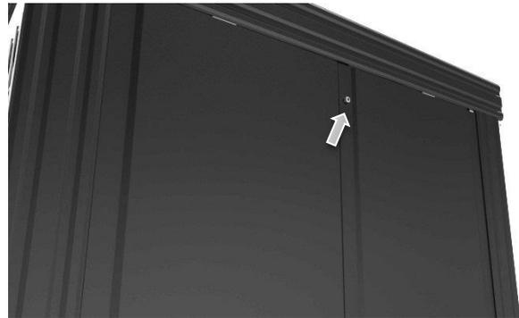
Use an Allan key n°5 with conical head to fix the back panels with screws and washers (torque of 3.5-4Nm).
