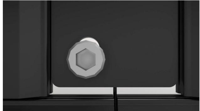
Use an Allan key n°5 with conical head to fix the back strip with screws and washers (torque of 3.5-4Nm).
