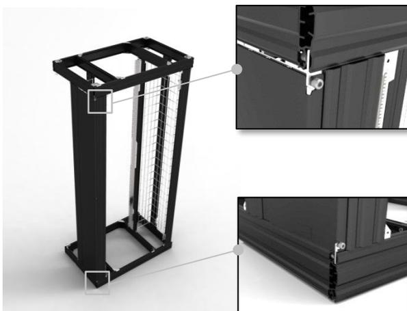
Use an Allan key n°5 with conical head to fix the side panel with screws and washers (torque of 3.5-4Nm).
