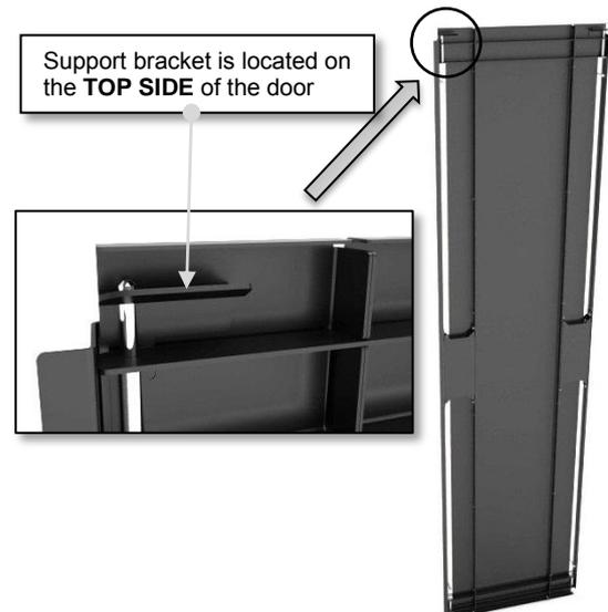
Support bracket is located on the TOP SIDE of the door
