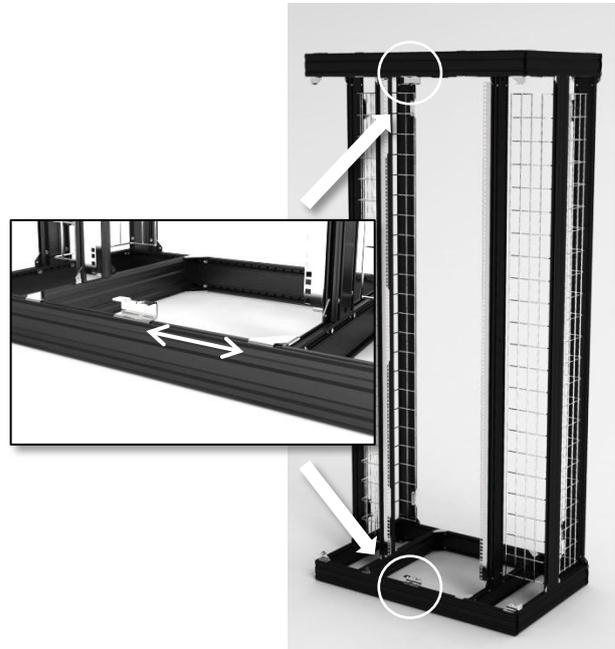
Assemble both hinge brackets with screws and washers in the middle of the horizontal profiles on the front side of the frame
