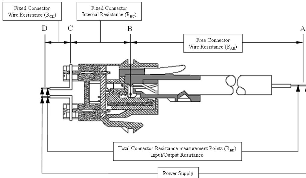
Jack-plug interface resistance:  $R_I = R_B = R_{AD} - (R_{AB} + R_{BD})$  [for reference only]
