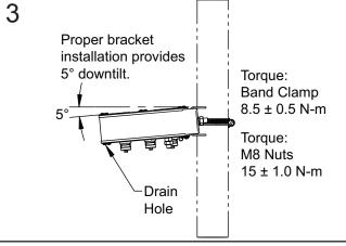
Ensure that junction box is properly mounted as shown. Torque M8 hardware and band clamp.
