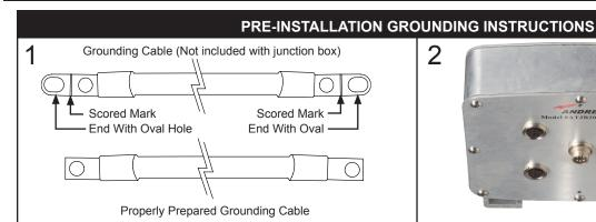
Break off both ends of the grounding cable, where the oval holes are located. This can be done by bending the tips at the scored marks.
