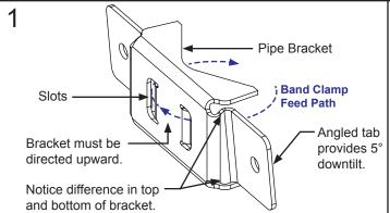
Note proper pipe bracket orientation. Insert band clamp through slots, positioning locking clasp so that it will be placed down behind the pipe.
