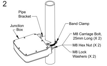
Attach band clamp to pipe.
