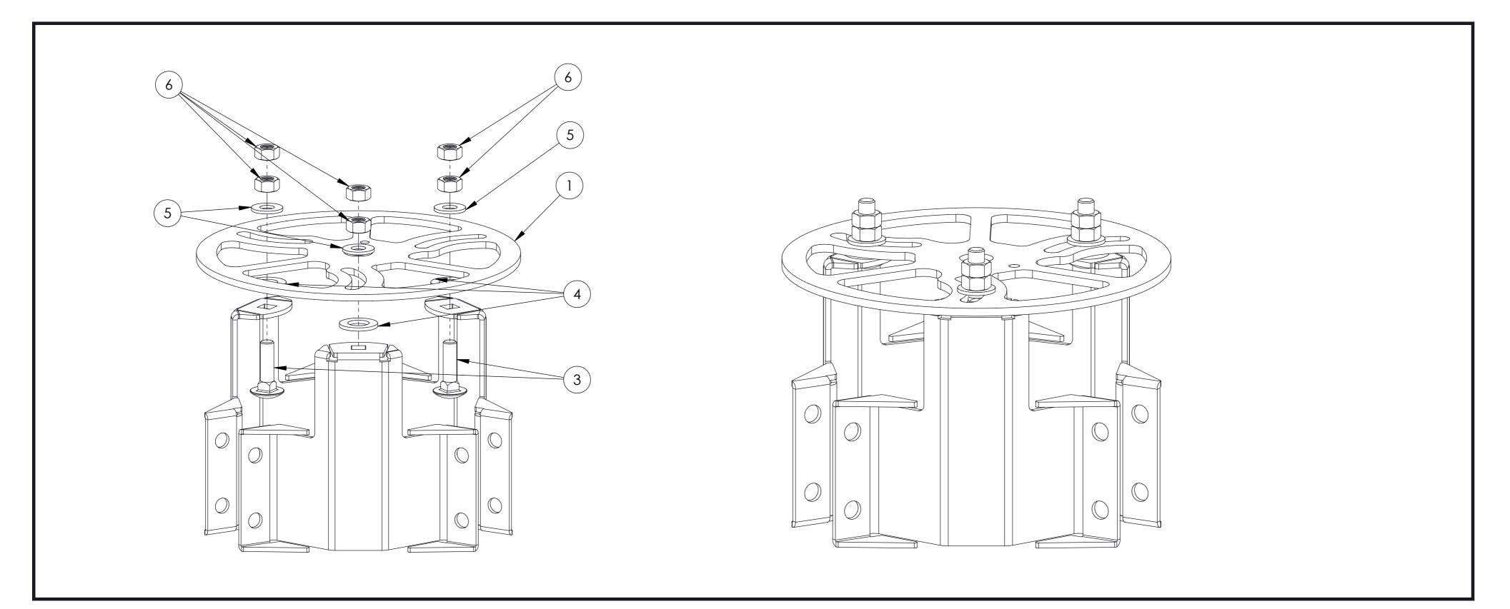
ASSEMBLE TOP MOUNT BRACKET TO PIPE MOUNT BRACKETS
