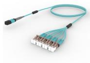
Ultra Low Loss OM4 MPO12 QSFP Unpinned to LC/UPC 8-Fiber InstaPATCH® 360 Ruggedized Fanout Cable, Low Smoke Zero Halogen
