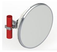
0.9m | 3 ft ValuLine® High Performance Low Profile Antenna, single-polarized, 5.925–7.125 GHz, CPR137G flange, white antenna, composite broadband grey radome without flash, standard pack—one-piece reflector
