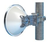
0.3 m | 1 ft ValuLine® High Performance Low Profile Antenna, dual-polarized, 14.250 – 15.350 GHz, PBR140 flange, white antenna, gray radome without flash, standard pack—one-piece reflector
