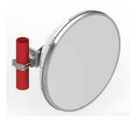
0.9m | 3 ft ValuLine® High Performance Low Profile Antenna, dual-polarized, 10.125–11.700 GHz, PDR100 flange, white antenna, composite broadband gray radome without flash, standard pack—one-piece reflector
