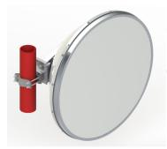
0.9m | 3 ft ValuLine® High Performance Low Profile Antenna, dualpolarized, 24.250–26.500 GHz, PBR220 flange, white antenna, composite broadband grey radome without flash, standard pack—onepiece reflector
