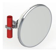
0.9m | 3 ft ValuLine® High Performance Low Profile Antenna, dual-polarized, 7.100–8.500 GHz, PBR84 flange, white antenna, composite broadband grey radome without flash, standard pack—one-piece reflector
