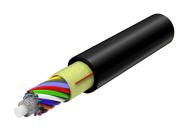
Fiber indoor/outdoor cable, LSZH, 12 fiber Microsheath, Tube Colours as per DIN/VDE 0888, Singlemode G.657.A1, Gel-free, Meters jacket marking, Black jacket color, Dca flame rating
