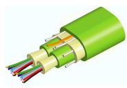
Fiber indoor cable, LazrSPEED® Low Smoke Zero Halogen Riser MPO Trunk, 24 fiber with 12 fiber 2.0mm subunits, Gel-free, Multimode OM5, Feet jacket marking, Lime green jacket color, B2ca flame rating
