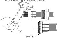
Cut off the redundant braid as shown.
