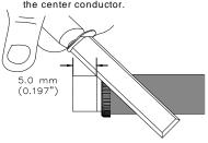
Make the braid small and sharp at the front; Slide part B and Screw part A onto cable without damaging the braid.
