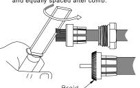
Cut off the redundant braid as shown.
