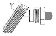
The cable center conductor must be straight and aligned with the connector inner contact. Insert the cable into the connector body until stopped: the center conductor must be inserted into the connector inner contact fingers. Tighten the connection to the torque value of 60-80 lb-in (6.8-9.0 N.m).
