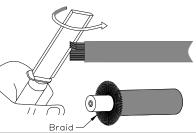
Remove 5.0 mm (0.197") of foam. Remove all foam/glue residue from the center conductor.
