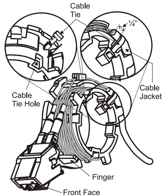
7. The spool adapter assembly is now ready for installation. Position the assembled spool adapter so that the front face is parallel and in line with the bottom hole (position 3) in the faceplate.
