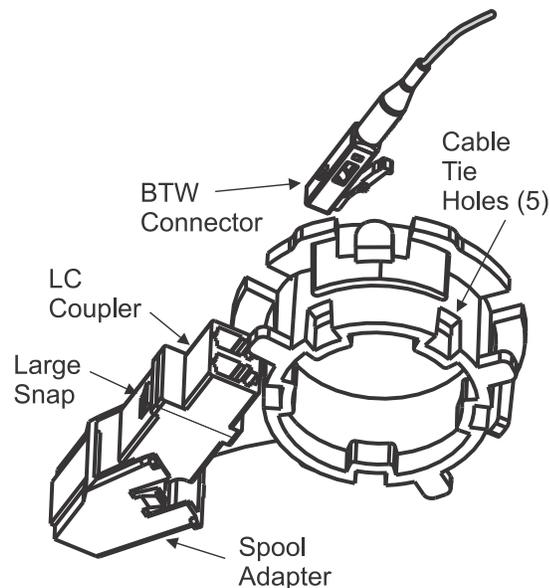
3. Begin winding the excess fiber so the first turn is positioned across the top of the guide and tucked under the guide post.
