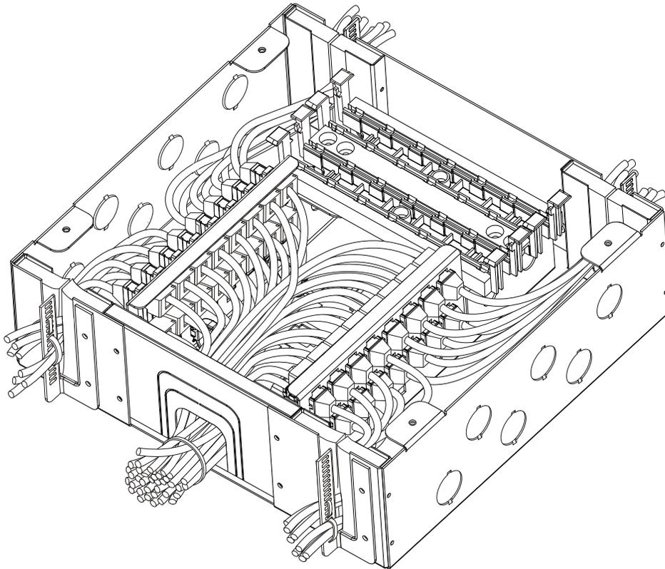
**Figure 4 — M32CPP Consolidation Point Box With Modules and Cables**
