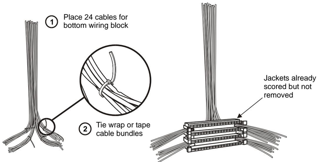
**NOTE:** M32CPP Consolidation Box not shown so cable routing can be seen.
