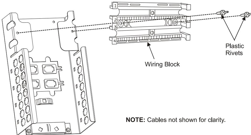
**Figure 6 — 110 Wiring Block Installation**
