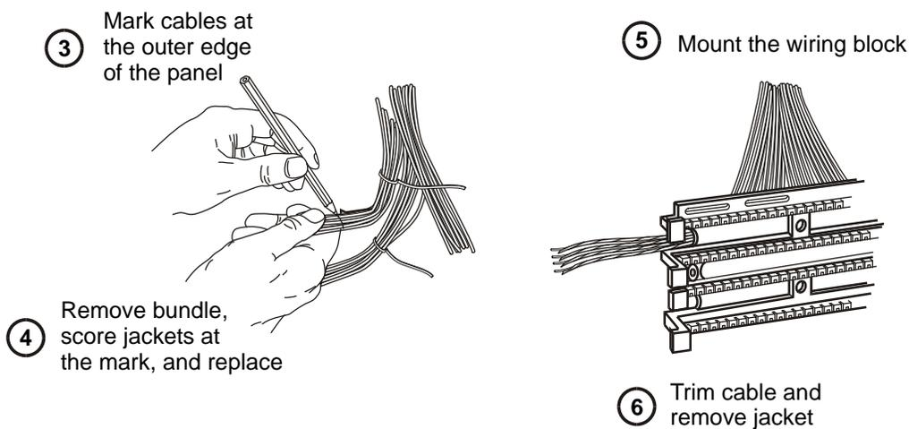
**Figure 7 — 110 Patch Panel Installation and Cable Routing**
