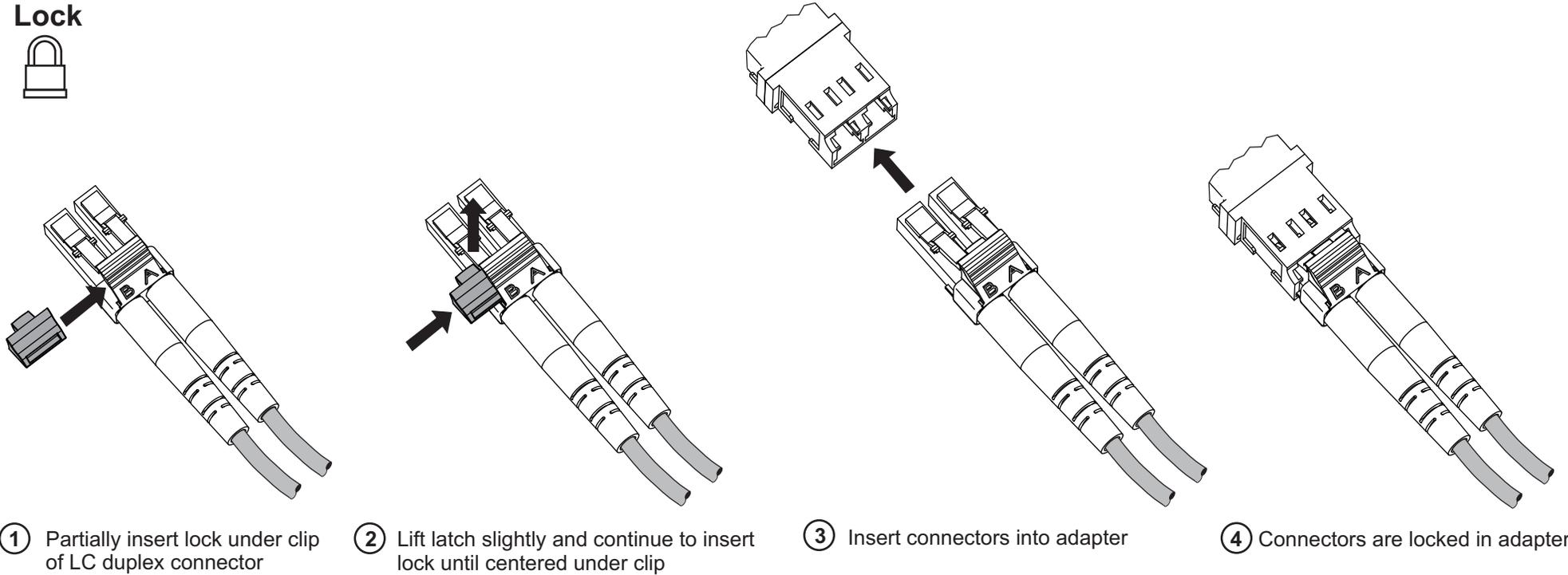
① Partially insert lock under clip of LC duplex connector
