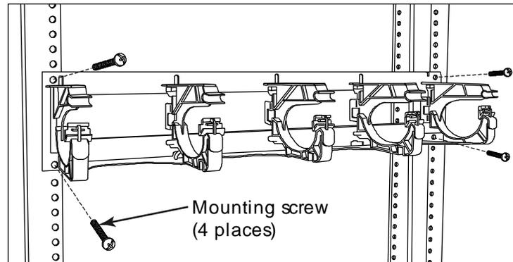
1. Using four screws (included), attach panel to 19-inch rack.
