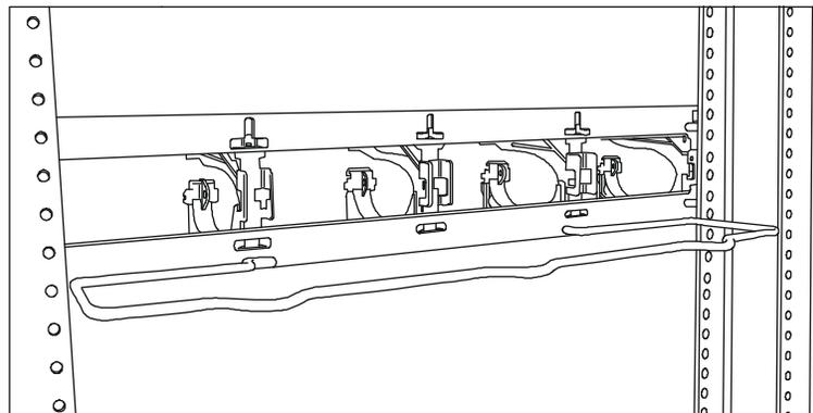
2. Install retainer bar to rear of panel.
