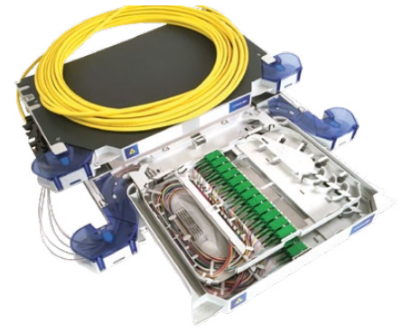
Figure 9: Two-element pre-cabled chassis with 96f. indoor microsheet cable and right-side patching
