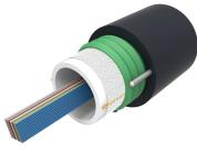
Fiber OSP cable, Steel Armored, Gel-Filled Central Tube Ribbon, 864 fiber, Singlemode G.652.D and G.657.A1, Feet jacket marking, Black jacket color
