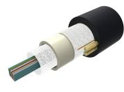
Fiber indoor/outdoor Cable, LSZH Riser All-Dielectric Central Tube Ribbon, Singlemode G.652.D and G.657.A1, 48-fiber, feet jacket marking, black jacket color
