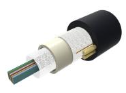
Fiber indoor/outdoor Cable, LSZH Riser All-Dielectric Central Tube Ribbon, Singlemode G.652.D and G.657.Al, 60-fiber, feet jacket marking, black jacket color
