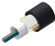
Fiber OSP Cable, Non-Armored, All-Dielectric, Gel-Filled Central Tube Ribbon, 36 fibers, Singlemode G.652.D and G.657.A1, Feet jacket marking, Black jacket color
