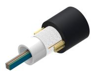
Fiber OSP Cable, Non-Armored, All-Dielectric, 864 fiber, Gel-Filled Central Tube Ribbon, Singlemode G.652.D and G.657.A1, Feet jacket marking, Black jacket color
