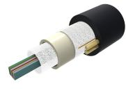
Fiber OSP Cable, Non-Armored, All-Dielectric, 144 fiber, Arid-Core, Dry Central Tube Ribbon, Singlemode G.652.D and G.657.A1, Gel-free, Feet jacket marking, Black jacket color
