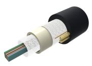
Fiber OSP Cable, Non-Armored, All-Dielectric, 192 fiber, Arid-Core, Dry Central Tube Ribbon, Singlemode G.652.D and G.657.A1, Gel-free, Feet jacket marking, Black jacket color
