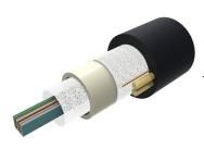
Fiber OSP Cable, Non-Armored, All-Dielectric, Arid-Core, 360 fiber, Dry Central Tube Ribbon, Singlemode G.652.D and G.657.A1, Gel-free, Feet jacket marking, Black jacket color
