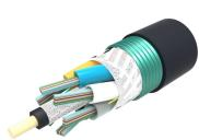
Fiber OSP cable, Steel Armored, Gel-Filled Loose Tube Ribbon, 432 fiber, Singlemode G.652.D and G.657.A1, Feet jacket marking, Black jacket color
