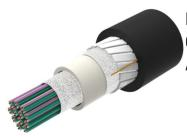
Fiber indoor/outdoor cable, All-Dielectric, LSZH Riser-Rated, 144 fiber, Gel-Free, Central Tube Rollable Ribbon, Singlemode G.652.D and G.657. Al, Feet jacket marking, Black jacket color, Cca flame rating
