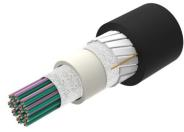
Fiber indoor/outdoor cable, All-Dielectric, LSZH Riser-Rated, Gel-Free, Central Tube Rollable Ribbon, 288 fiber, Singlemode G.652.D and G.657. Al, Feet jacket marking, Black jacket color, Cca flame rating
