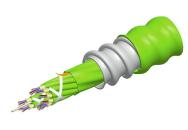
Fiber indoor cable, LazrSPEED® Riser/LSZH rated, MPO Trunk, interlocking aluminum armored, Multimode OM5, 24 fiber, Feet jacket marking, Lime-green jacket color, B2ca flame rating
