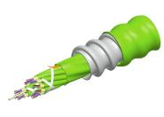
Fiber indoor cable, LazrSPEED® Riser/LSZH rated, MPO Trunk, interlocking aluminum armored, Multimode OM5, 96 fiber, Feet jacket marking, Lime-green jacket color, B2ca flame rating
