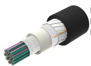
Fiber OSP cable, Non-Armored, All-Dielectric, Arid-Core, Dry Central Tube Rollable Ribbon, 144 fiber, Singlemode G.652.D and G.657.A1, Gel-free, Feet jacket marking, Black jacket color
