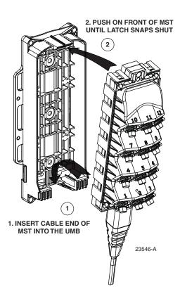
Figure 11. Installing the MST in the Universal Mounting Bracket
