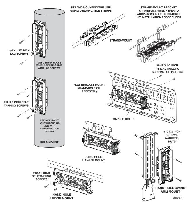
Figure 10. Typical Installation of a Universal Mounting Bracket (UMB)
