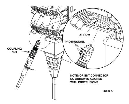
Figure 15. Typical Connection of a Drop Cable To MST Optical Port
