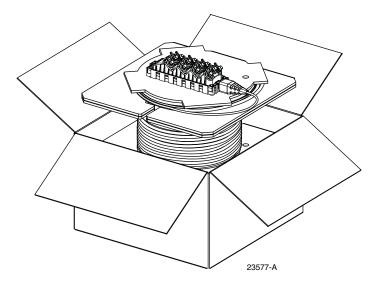
Figure 5. Typical Distribution Cable on a Spool
