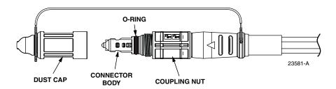
Figure 13. Drop Cable Connector Components
