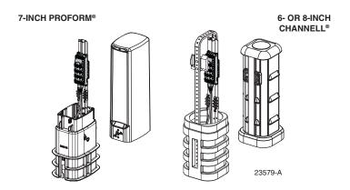
Figure 7. Typical Pedestal Mounting
