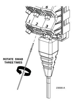
Figure 19. Typical Cleaning of an Optical Port Connector and Adapter
