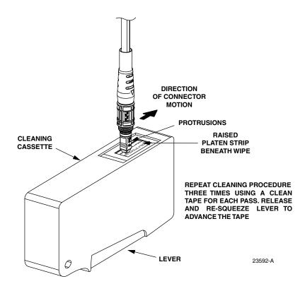
Figure 18. Cleaning Drop Cable Connector
