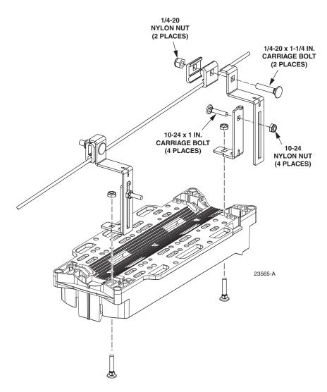
Figure 12. Securing Strand-Mounted MST
