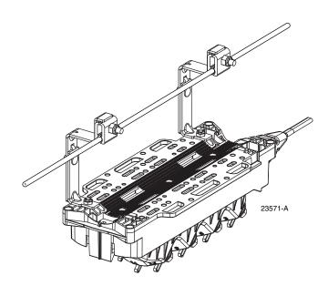
Figure 9. Typical Strand-Mount Installation
