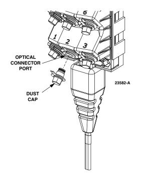
Figure 14. Typical Optical Port Adapter Components
