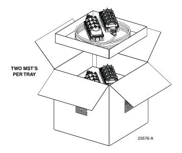
Figure 4. Typical MST Cable Coiled and MST Placed in a Box
