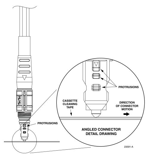
Figure 17. Typical Angled Connector End-Face Detail
