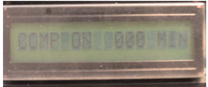
Mode 2: Displays pressure and total run hours, flashes current condition.
