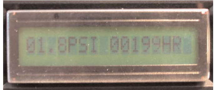
Mode 1: Displays pressure and total run hours.
