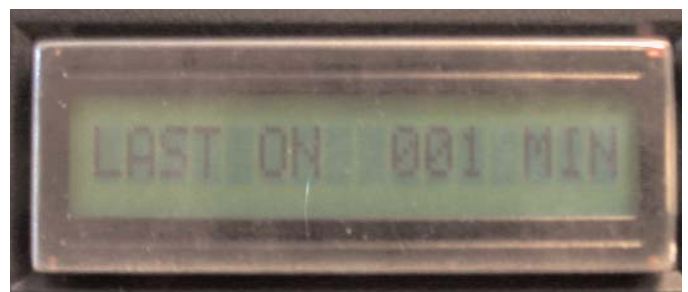
Mode 3: Displays last ON and last OFF times.
