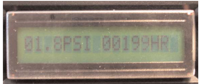
Mode 1: Displays pressure and total run hours.
