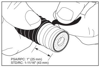
**4** Slit and peel the scored section of jacketing. Proceed to the connector installation bulletin.
