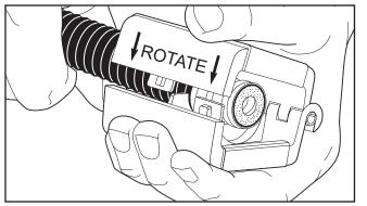
**3** Lightly squeeze the tool halves together and rotate the tool counterclockwise (as viewed from the cable end) approximately 12 revolutions until the cut section falls away. **Note:** Keep a constant grip on the tool. Do not release the tool during rotation because this may result in an uneven cut.
