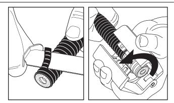
**2** Remove about 1.5" to 1.6" (38 to 40 mm) of the jacket from the cable end by scoring and slicing the jacket. Position the tool on the cable so that the corrugation guide is about 1-1/4" (32 mm) from the cable end (usually the first corrugation root available adjacent the cable jacket).
