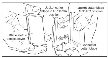
1 Check to be sure that the jacket cutter blade is in the correct position for the connector type -- STD/RC or RPC -- to be attached to the prepared cable. To change the blade position, pull off the blade slot access cover and insert the blade in the desired position and replace the cover.
