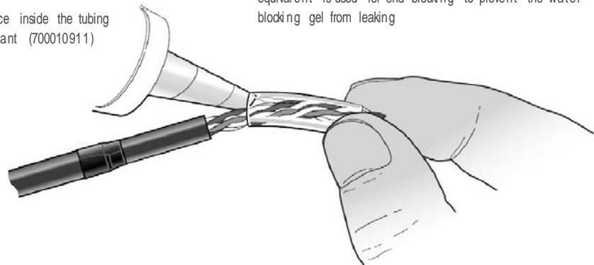
Position the filled tube to overlap the end of the inner jacket
