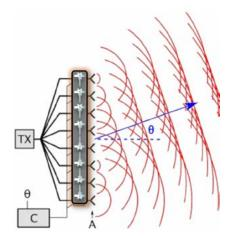
Figure 14: Effect of phase shift
