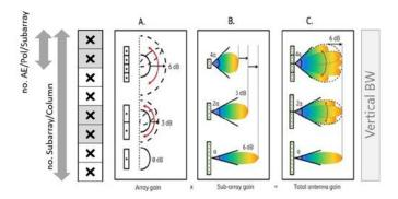
Figure 12: Subarrays gain, modified from [8]
