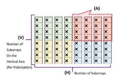
Figure 35: Antenna panel dimensions
