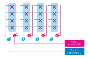
Figure 31: Beamforming with four-column antenna
