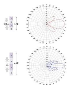
Figure 13: Antenna elements spacing effect
