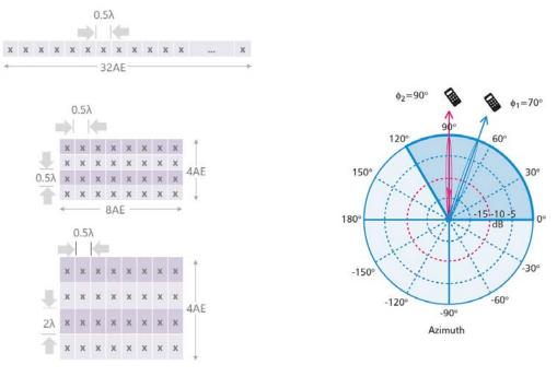
Figure 37: 64T64R mMIMO panel configuration
