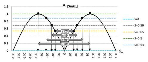
Figure 21: Column spacing vs. max scan angle
