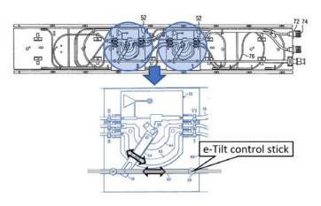
Figure 15: CommScope patented e-tilt phase shifters
