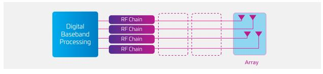
Figure 17: Digital beamforming
