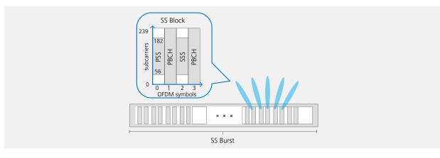
Figure 1: Directional SS blocks transmission
