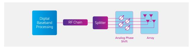
Figure 16: Analog beamforming
