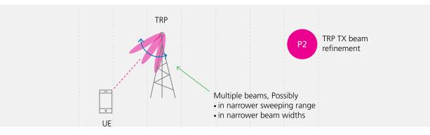
Figure 6: DL Tx beam refinement [6]
