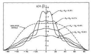
Figure 20: Element spacing vs HP-HBW [12]
