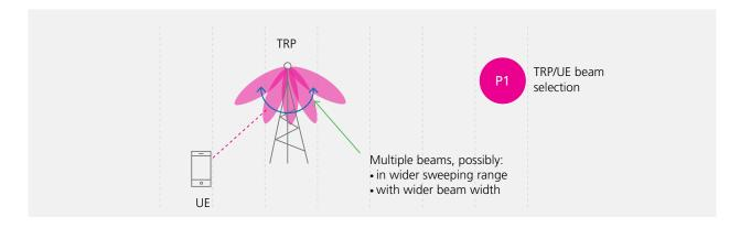
Figure 5: DL Tx beam selection [6]
