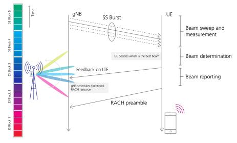
Figure 2: Initial access in NSA mode [3]
