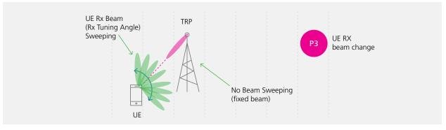
Figure 7: DL Rx beam refinement [6]
