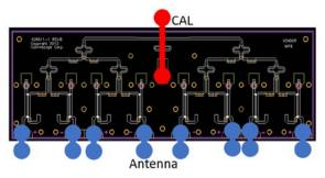
Figure 28: Calibration board
