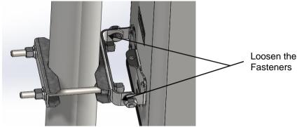
Figure 9: Lower Mounting Bracket Assembly
