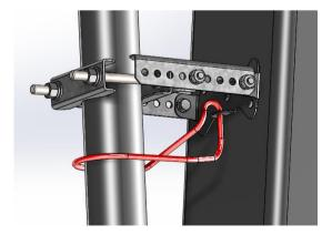
Figure 8: Upper Mounting Bracket Assembly
