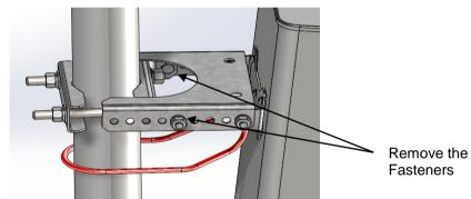
Figure 10: Upper Mounting Bracket Assembly
