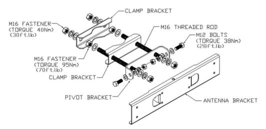
Figure 3: Exploded Assembly for Lower Mounting Bracket using Clamp Bracket (This configuration should also be used for the upper Mounting Bracket when 0° tilt is required)
