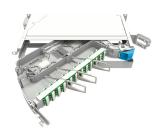
MFPS Fiber Optic panel, 1RU, 48 fibers/RU, splice/patch, SMOUV/front patch cords orientation to the right, 12 SC/APC, grade C
