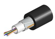
Fiber OSP cable, PE, Gel-filled Central Tube, 6 fiber, Singlemode G.652.D and G.657.A1, Meters jacket marking, Black jacket color
