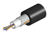
Fiber OSP cable, PE, Gel-filled Central Tube, All-dielectric, 6 fiber, Multimode OM3, Meters jacket marking, Black jacket color
