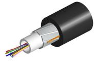
Fiber OSP cable, PE, Gel-filled Central Tube, All-dielectric, 12 fiber, Multimode OM3, Meters jacket marking, Black jacket color
