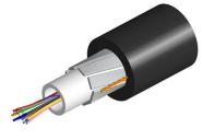
Fiber OSP cable, PE, Gel-filled Central Tube, All-dielectric, 24 fiber, Multimode OM3, Meters jacket marking, Black jacket color
