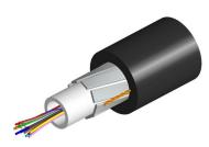
Fiber OSP cable, PE, Gel-filled Central Tube, All-dielectric, 12 fiber, Multimode OM4, Meters jacket marking, Black jacket color
