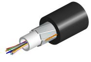
Fiber OSP cable, PE, Gel-filled Central Tube, All-dielectric, 24 fiber, Multimode OM4, Meters jacket marking, Black jacket color
