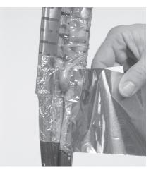
9 Apply a new aluminium cable foil over the existing cable bundle.
