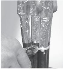
8 Remove the tie-wrap from the cable bundle.
