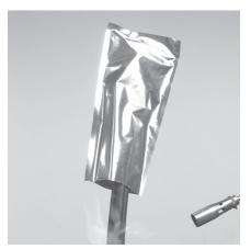
8 **For PEDCAP-R-3 and PEDCAP-R-4S/4L** temporarily position the aluminium bag over the joint to protect joint and conductors from damage (flame protection). Do not tape. Flame brush the abraded area of each cable for 10 seconds.
