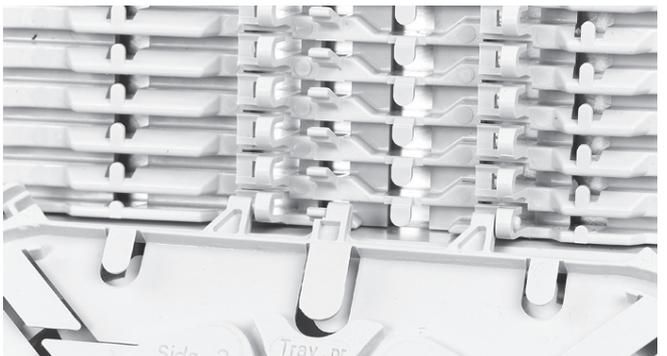
4.4 Place a tray in the wraparound groove plate; do this by pushing the lip on the groove plate (lowest possible position) slightly down with the tray and move the tray lateral into the hinge-cavities of the groove plate. To snap the High Capacity Single Element tray (HCSE) in the W/a single fiber groove plate leave always one hinge facility open between Fasblock or previous tray and the HCSE-tray.
